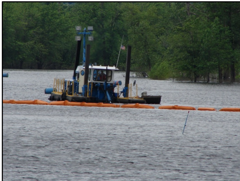
Photograph M-2: Small Hydraulic Dredge (Lake Odessa HREP Stage IIA)
